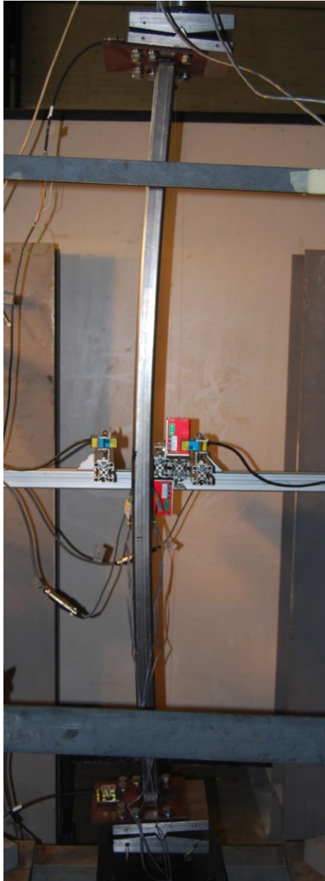
Figure 8. Overall flexural buckling failure of specimen S3-EC1.
