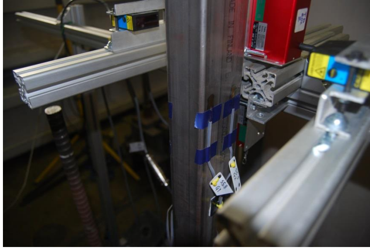
Figure 7. In detail instrumentation setup at mid-height section.
