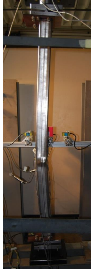
Figure 9. Interaction of local and overall flexural buckling of specimen S4-CC.
