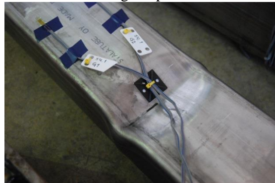
Figure 10. Detailed view of the local failure of specimen S4-EC1.
